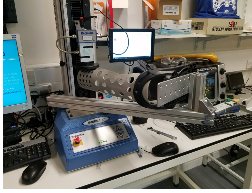
Figure 15: The setup used for the bend test with the Mecmesin force tester.
